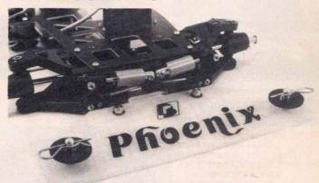
REAR SUSPENSION COMPON-ENTS ARE DIRECTLY MOUNTED TO THE ALLOY 7075-T6 SIDEPLATES FOR MAXIMUM RIGIDITY AND STRENGTH.
