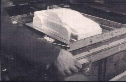
Below: An F1 shell ready to be removed from the mould as soon as the temperature comes down.
