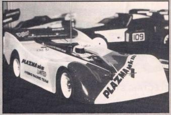
Scene at the recent Nuremburg Toy and Hobby Fair was this new Kyosho 1/12 car. The "Plazma Mk ??" is produced from high quality carbon sheet and nicely machined aluminium components. The car also "Features rear suspension via a single Option House" gold off road damper. As to whether the car would go into production – we don't know, but if it does it should go well
