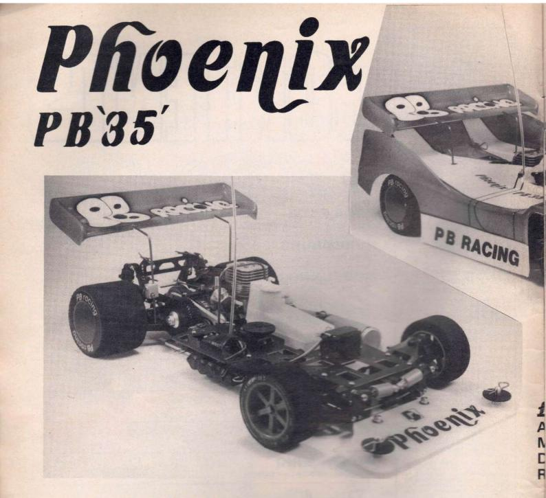
THE PHOENIX HAS BEEN DEVELOPED TO PROVIDE YOU WITH A COMIC CAR AT A VERY COMPETITIVE PRICE BUT WITH STRENGTH AND FUNIQUE TWO BELT, FOUR WHEEL DRIVE SYSTEM WILL ABSORBLESS POWNHEELS. "THE 22 KEVLAR COMPOSITE" FRONT DRIVE BELT HAS BEEN POUNDS BREAKING STRAIN AND OFFERS LOW FRICTION AND WEAR MANUFACTURED FROM THE FINEST AEROSPACE ALLOY 7075-T6. FOR SURADIO PLATE IS QUICKLY REMOVEABLE FOR CLEANING AND ITS 'EPOXY CONTROL CONSTRUCTION.
